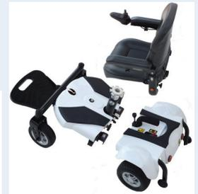
Dismantles easily into 3 pieces to fit in a car boot for transportation
